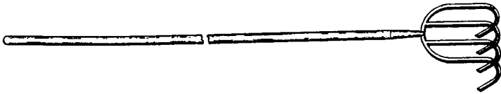
Rake for taking aquatic plants from ponds.
