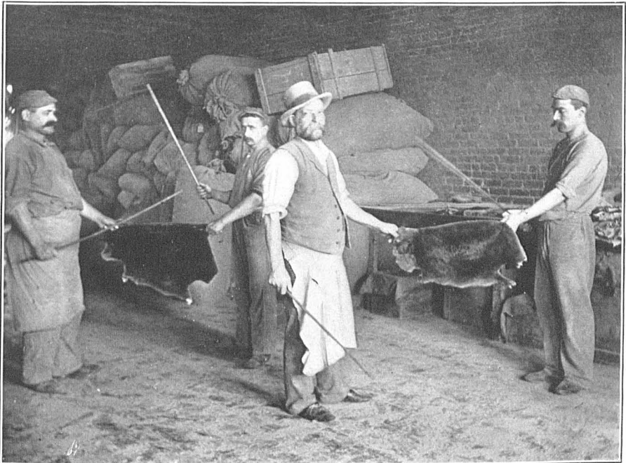
BEATING BEAVER SKINS FOR REMOVING SAWDUST, ETC.
