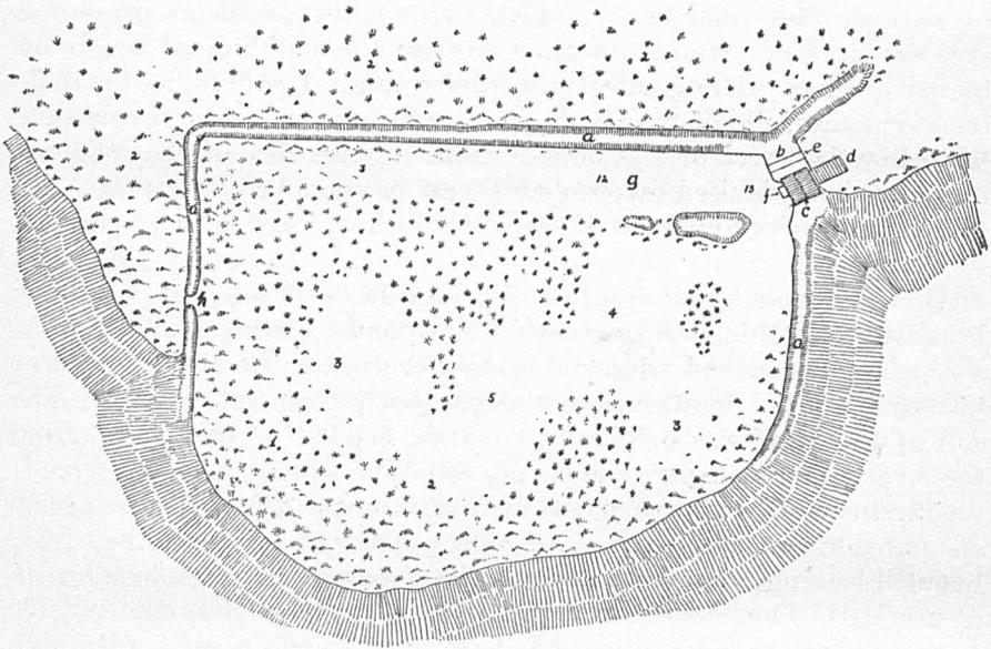
Diagrammatic plan of carp pond near Port Clinton, Ohio: *a*, embankment; *b*, dam; *c*, engine-house; *d*, water elevator; *e*, chute through which fish are slid into pond; *f*, chute through which fresh water enters pond; *g*, dredge-cut; *h*, outlet. The figures indicate depth of water.
