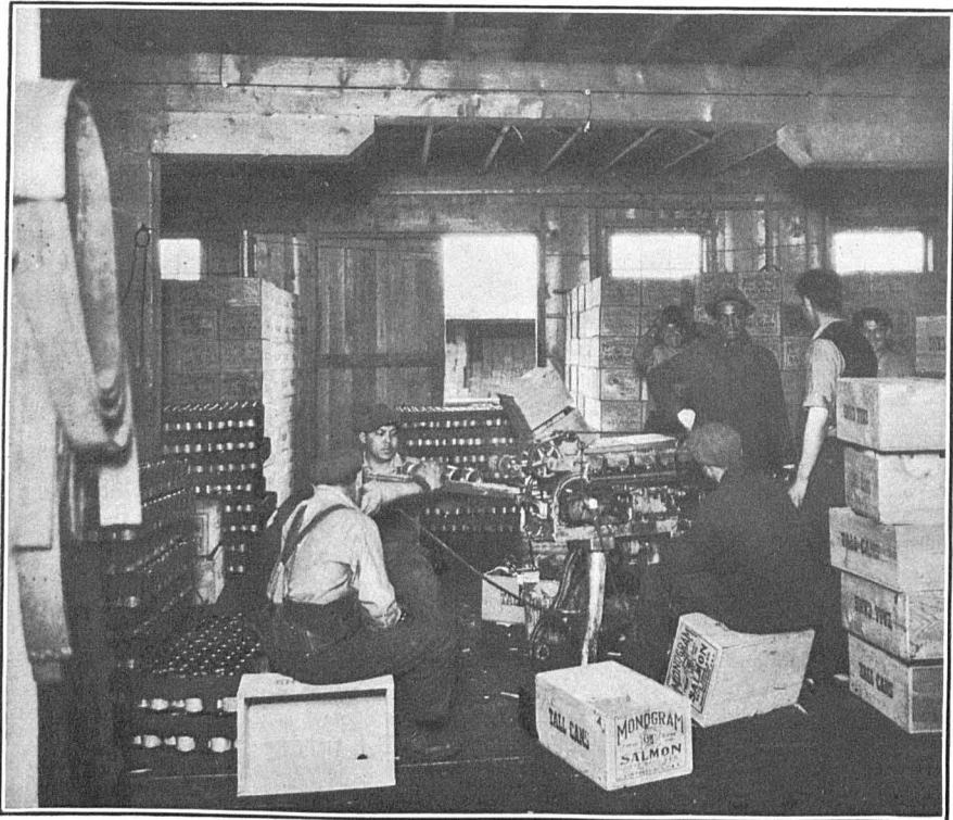
FIG. 2.—SALMON CAN-LABELING MACHINE:
