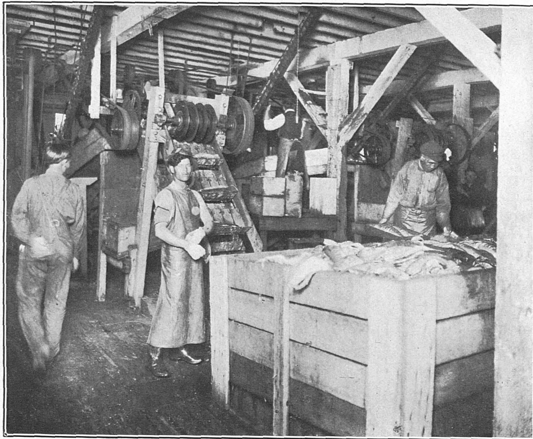
FIG. 29.—CUTTING SALMON INTO PIECES OF A SIZE TO FIT THE CAN.
