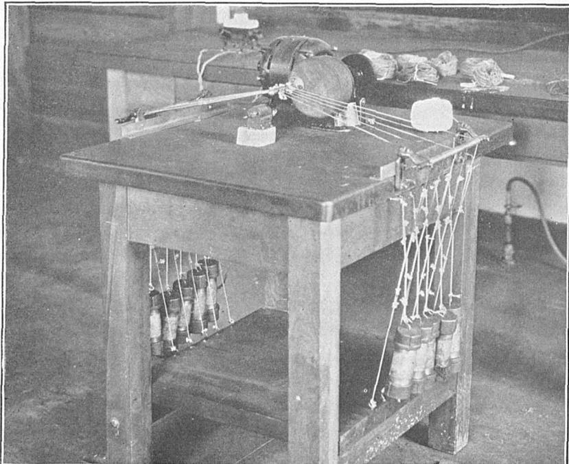
FIG. 9.—Machine used for making wearing tests.
