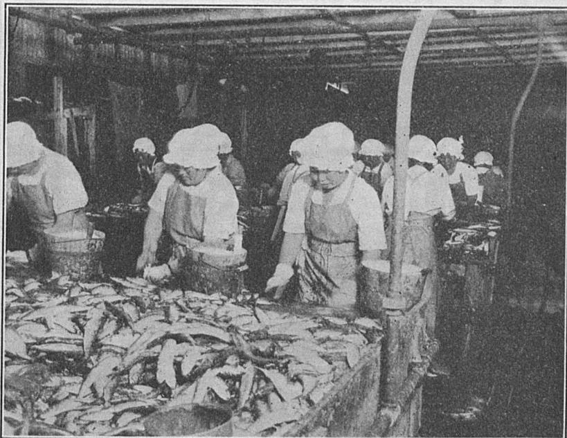
FIG. 3. Hand cutting. The fish from the holding tanks are flumed to tables as needed
