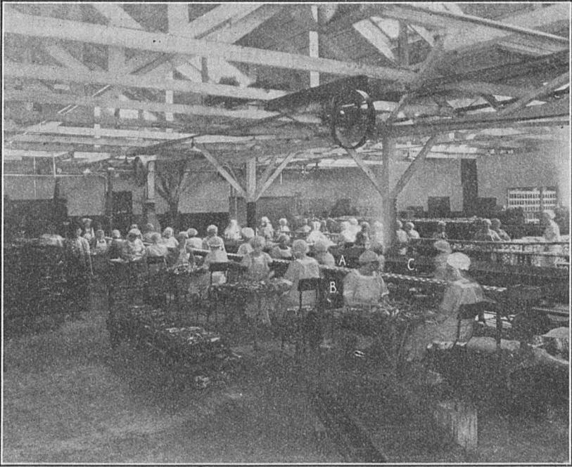
FIG. 13.—Packing. Men empty baskets of fish on the tables as needed. Cans with sauce in them are obtained from the upper conveyor A, and when filled are weighed and then placed on the lower conveyor B, which carried them to the sealing machines. C is the exhaust box shown in Figure 14
