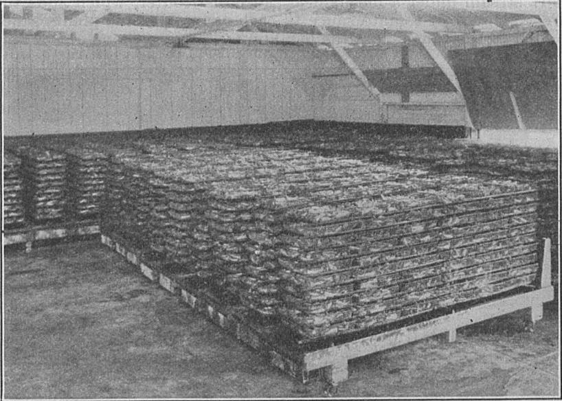
FIG. 11.—Cooling and draining. Large fish usually stand overnight for this purpose. Note containers at ends of trucks for catching oil and water draining from the fish
