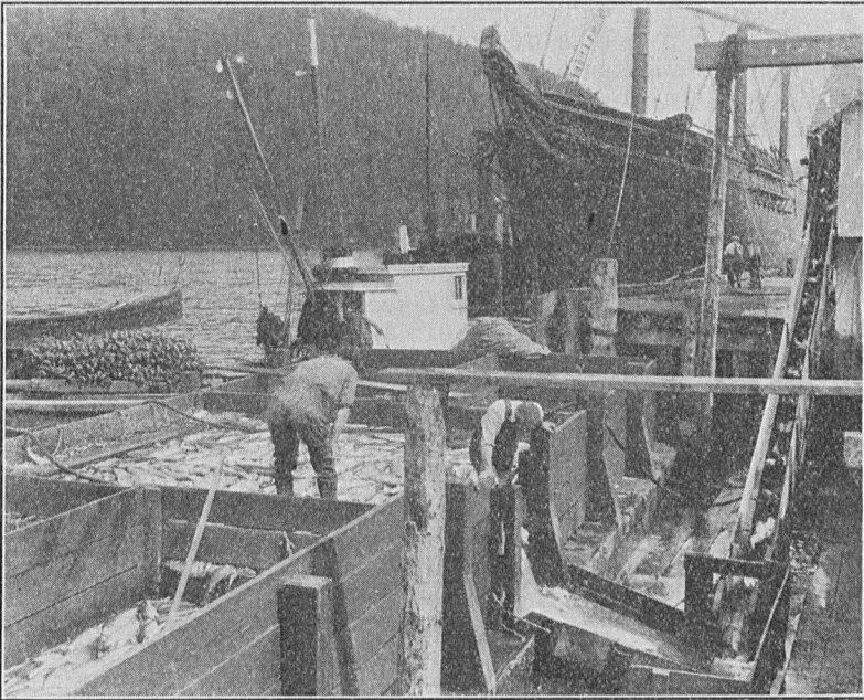
FIG. 7.—Sluicing salmon from lighter at cannery, southeast Alaska
