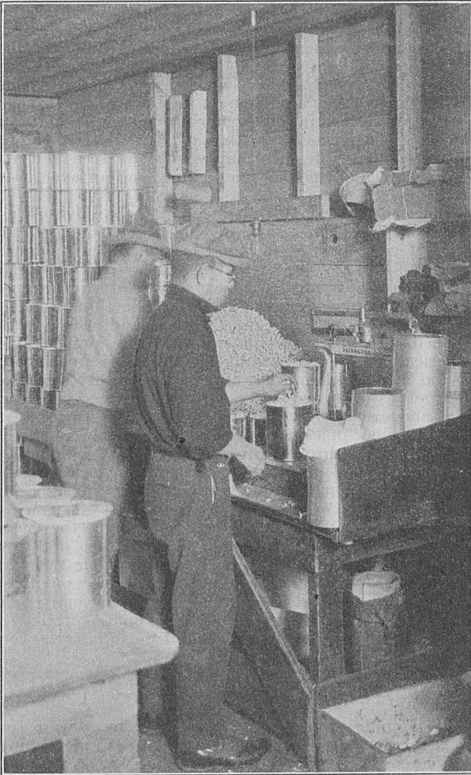
FIG. 8.—Weighing and packing the shrimp meat
