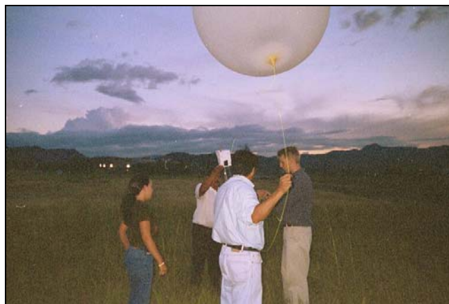
Upper Air System Balloon and Instrument Package
