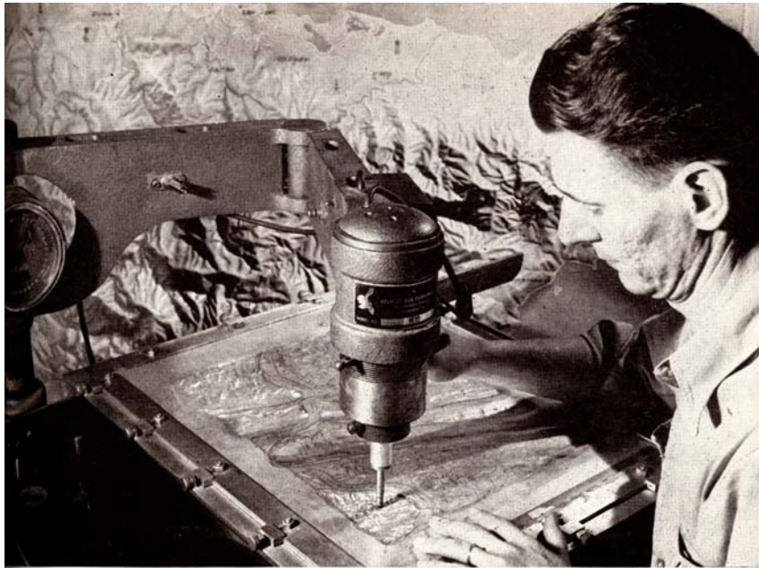
er model—a thin guage aluminum sheet—is formed on the Reliefograph. The “altimeter” is seen on the left.
