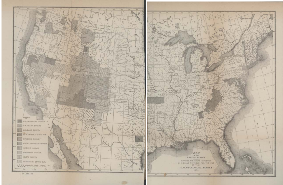
Areas of the US Suitable for topographic mapping by USGS map prepared by USGS, 1884 and submitted to the Allison Commission shaded areas had sufficient geodetic control for mapping
