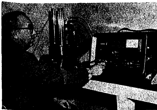
Fig. 30--Highly sensitive detection devices are used by the Radiobiological Laboratory to measure radioactivity present in fish and shellfish.
