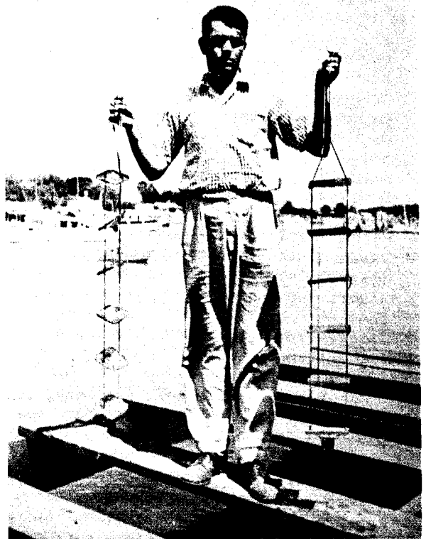
TESTING PLASTIC COLLECTORS TO SECURE OYSTER SET
