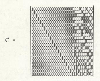
Figure 7. -- Systematic 21/31 BCH generator matrix.
