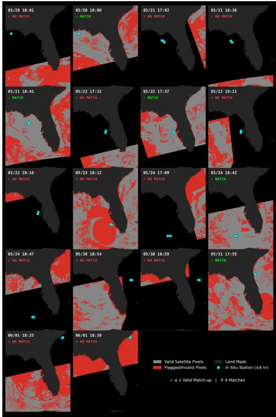
Figure 56. Evaluation of PACE-OCI Level-2 spatial coverage and in situ matchup potential. Panels display valid water pixels (grey), flagged/invalid pixels (red), and concurrent ( \pm 4 hours) in situ stations (cyan circles). Text indicators denote the successful presence ( \checkmark ) or absence ( \times ) of at least one valid spatial match-up for each orbital overpass.
