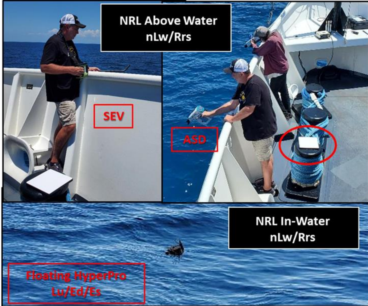
Figure 22. Pictures illustrate the above-water collection using the Spectral Evolution and ASD (top 2 pictures). The bottom picture illustrates the TSRB deployment.
