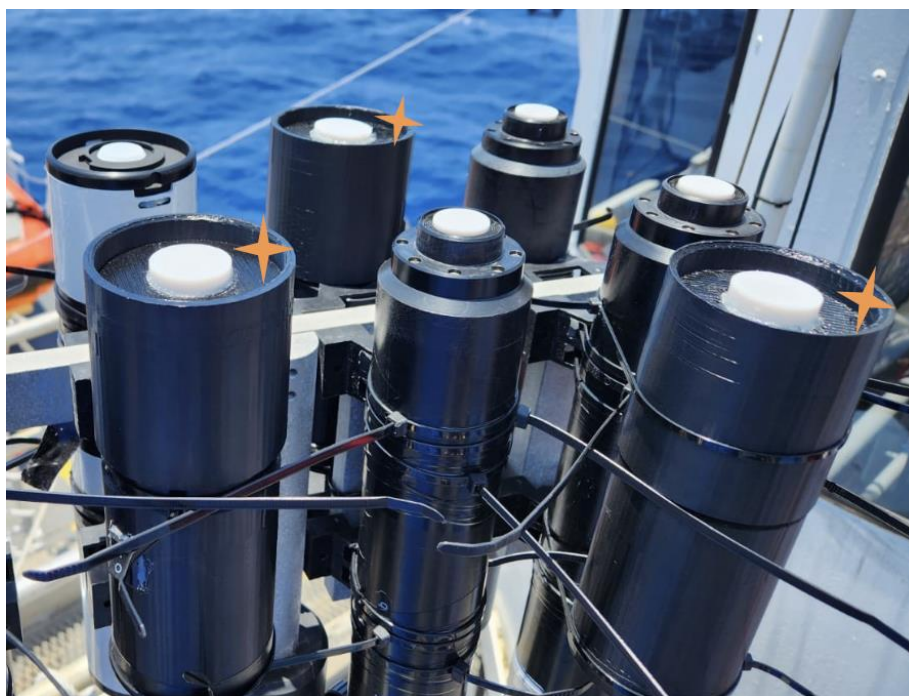
Figure 41. Open Source spectral sensors (3D-printed housings with die-cut PTFE cosine correctors) are marked with an orange star. They are mounted directly adjacent to HyperOCRs and a Biospherical irradiance sensor.
