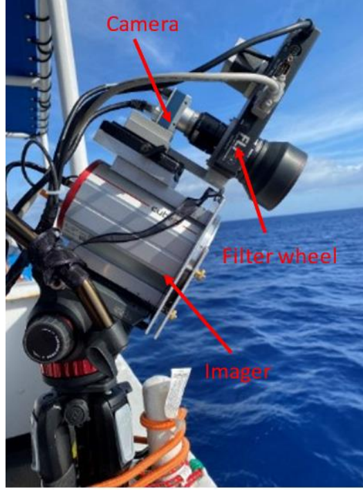
Figure 32. Snapshot hyperspectral imager with polarization camera on the ship.
