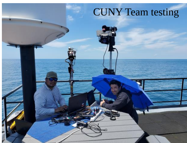
Figure 5. Above-water radiometric measurements conducted from the foredeck and upper deck of Nancy Foster (Clockwise from top-left: handheld radiometers measuring total radiance from the water surface; handheld radiometers measuring sky radiance; mounted DALEC radiometric system; mounted hyperspectral polarization camera systems).
