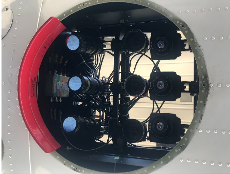
Figure 3. -- View of the mounted camera array from underneath the aircraft showing UV, color (RGB), and thermal cameras from left to right. The UV cameras were disabled for this project.
