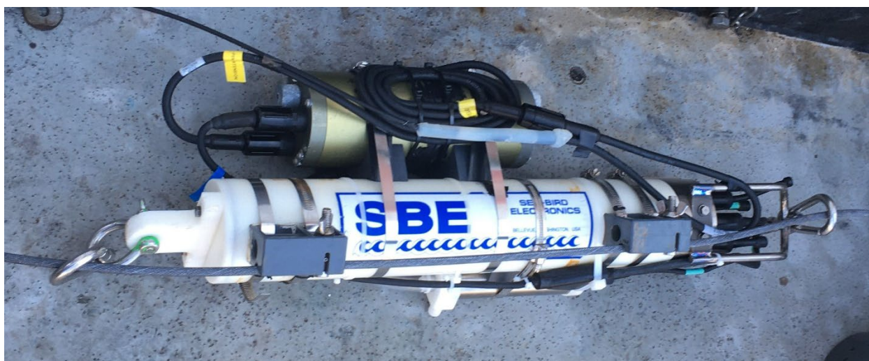
Figure 2: An SBE-19plusV2 SeaCat CTD on deck with attached pump and power and data interface module (PDIM). Photo Credit: Chris Taylor.
