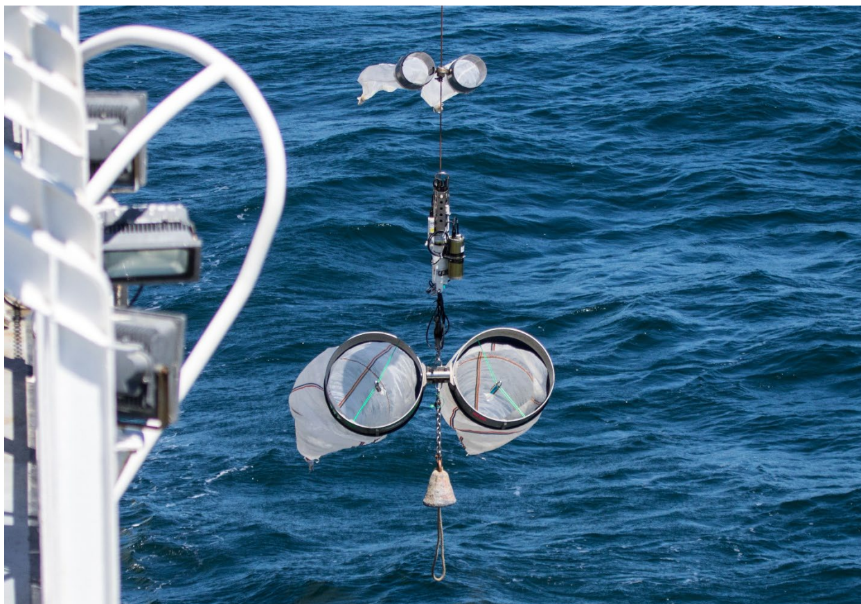
Figure 3: An SBE-19plus V2 CTD mounted with bongo nets and depressor weight for a double oblique towed deployment. Photo Credit: Chris Melrose.
