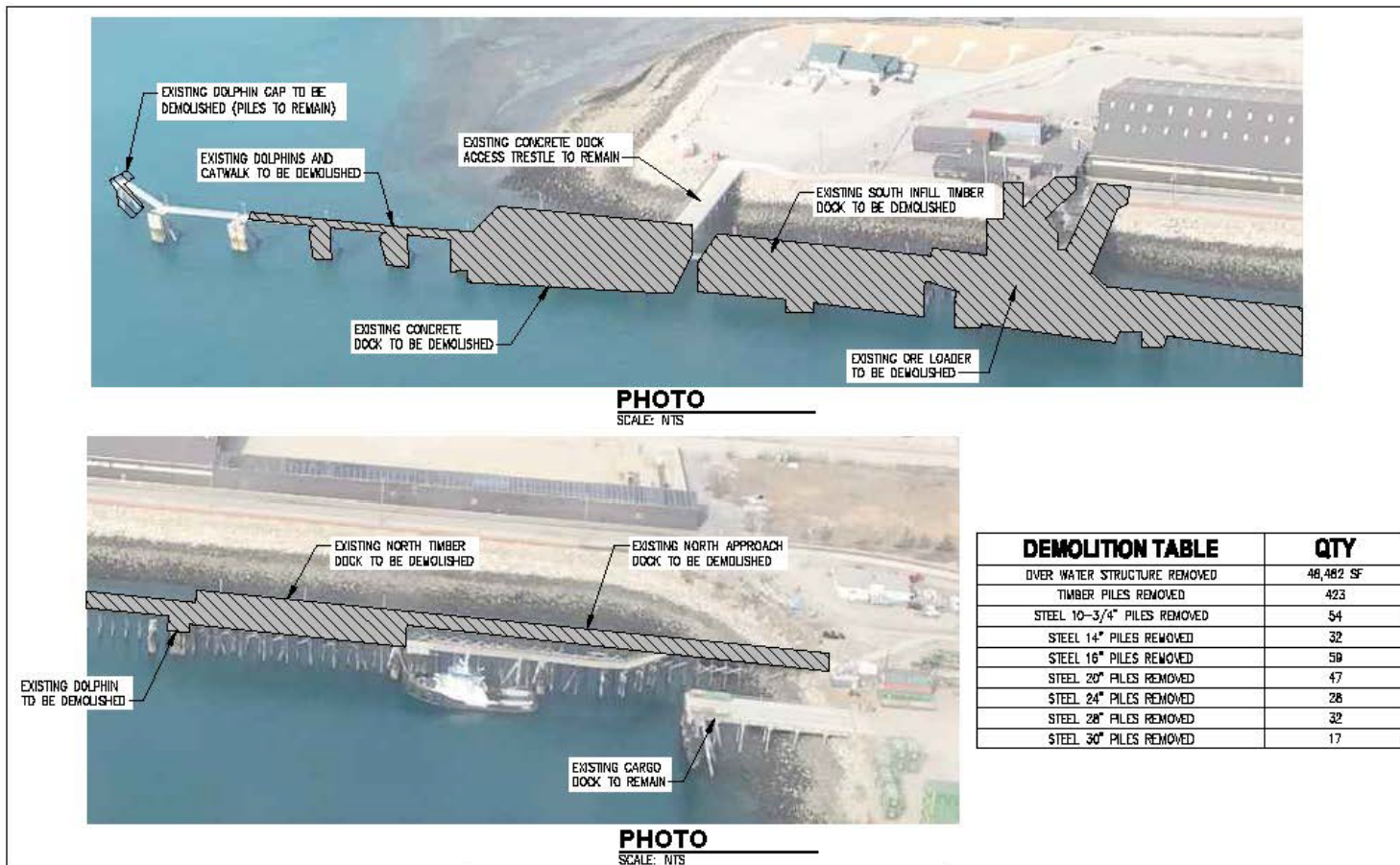
Figure 2. Existing Infrastructure at the Ore Terminal.
