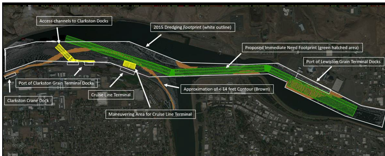
Figure 2. Federal Navigation Channel near Clarkston, WA and Lewiston, ID. Navigation channel is in green. Access channels are in yellow, and the shallow-water areas are in orange (USACE 2022).
