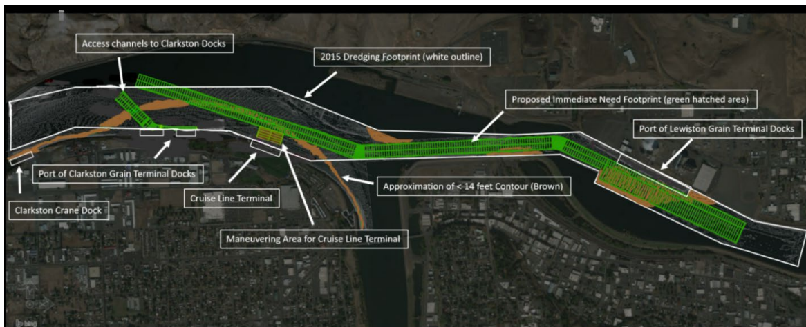
Figure 1. Proposed dredging regions outlined in green polygons. Main polygon includes the Clearwater River and downstream of the confluence, secondary polygon includes downstream portion in the Snake River.
