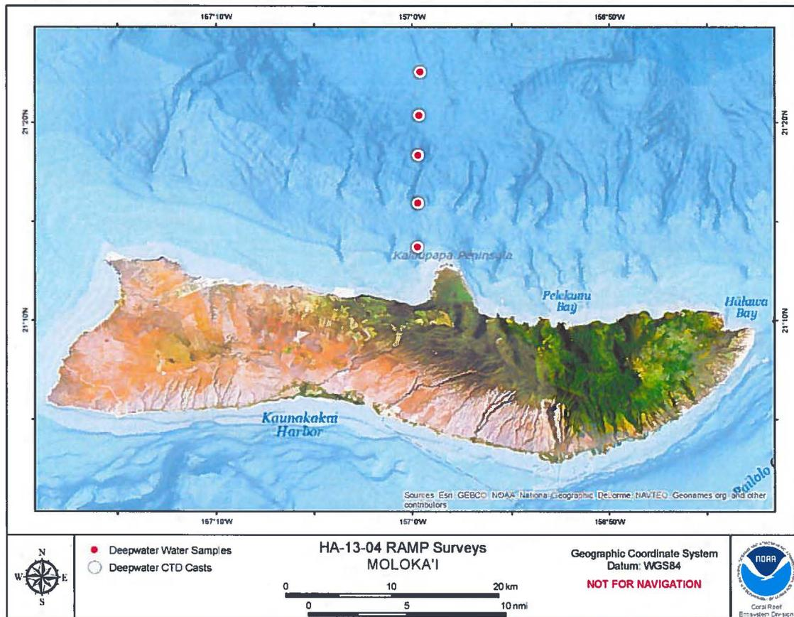
**Figure F.1.2.**--Locations of deep-water CTD casts and water sampling performed at Moloka`i Island during cruise HA-13-04. (Sources: Landsat satellite imagery data from the U.S. Geological Survey; bathymetry imagery data from Esri, GEBCO, NOAA, National Geographic, DeLorme, NAVTEQ, Geonames.org, and other contributors.)
