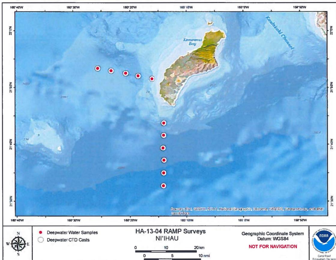
**Figure G.1.2.**--Locations of deep-water CTD casts and water sampling performed at Ni'ihau Island during cruise HA-13-04. (Sources: Landsat satellite imagery data from the U.S. Geological Survey; bathymetry imagery data from Esri, GEBCO, NOAA, National Geographic, DeLorme, NAVTEQ, Geonames.org, and other contributors.)
