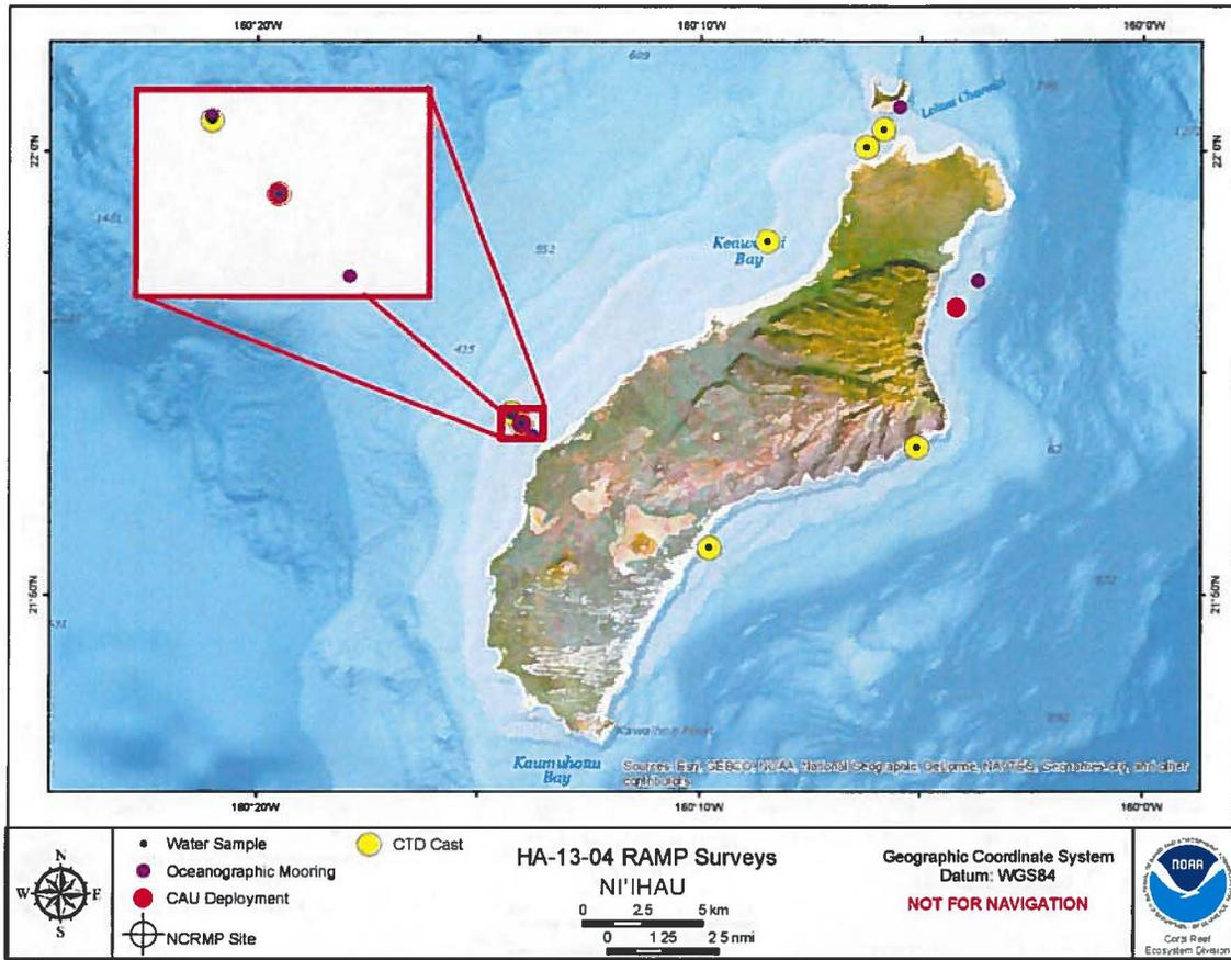
**Figure G.1.1.--**Mooring sites where oceanographic instruments and biological installations were retrieved or deployed and locations of nearshore CTD casts and water sampling performed at Ni'ihau Island and Lehua Rock during cruise HA-13-04. (Sources: Landsat satellite imagery data from the U.S. Geological Survey; bathymetry imagery data from Esri, GEBCO, NOAA, National Geographic, DeLorme, NAVTEQ, Geonames.org, and other contributors.)
