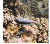
**Subsurface Temperature Recorders (STR)** are deployed on coral reefs in shallow water (<30 m) to measure water temperature. Temperature information provides insight into several water properties that affect coral reefs.
