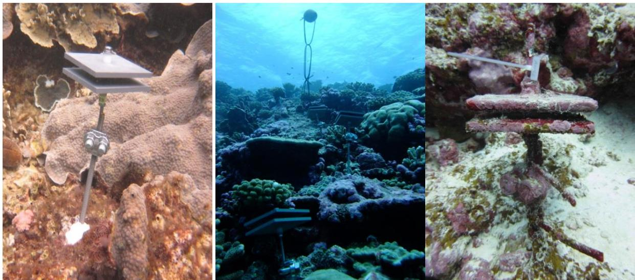
**Figure 114.** Newly deployed Calcification Accretion Unit (CAU) on the seafloor at one of the Climate Monitoring sites in Timor-Leste (*left*). CAUs installed within a Climate Monitoring site with an STR deployed nearby (*middle*). CAU about to be recovered approximately two years later (*right*).
