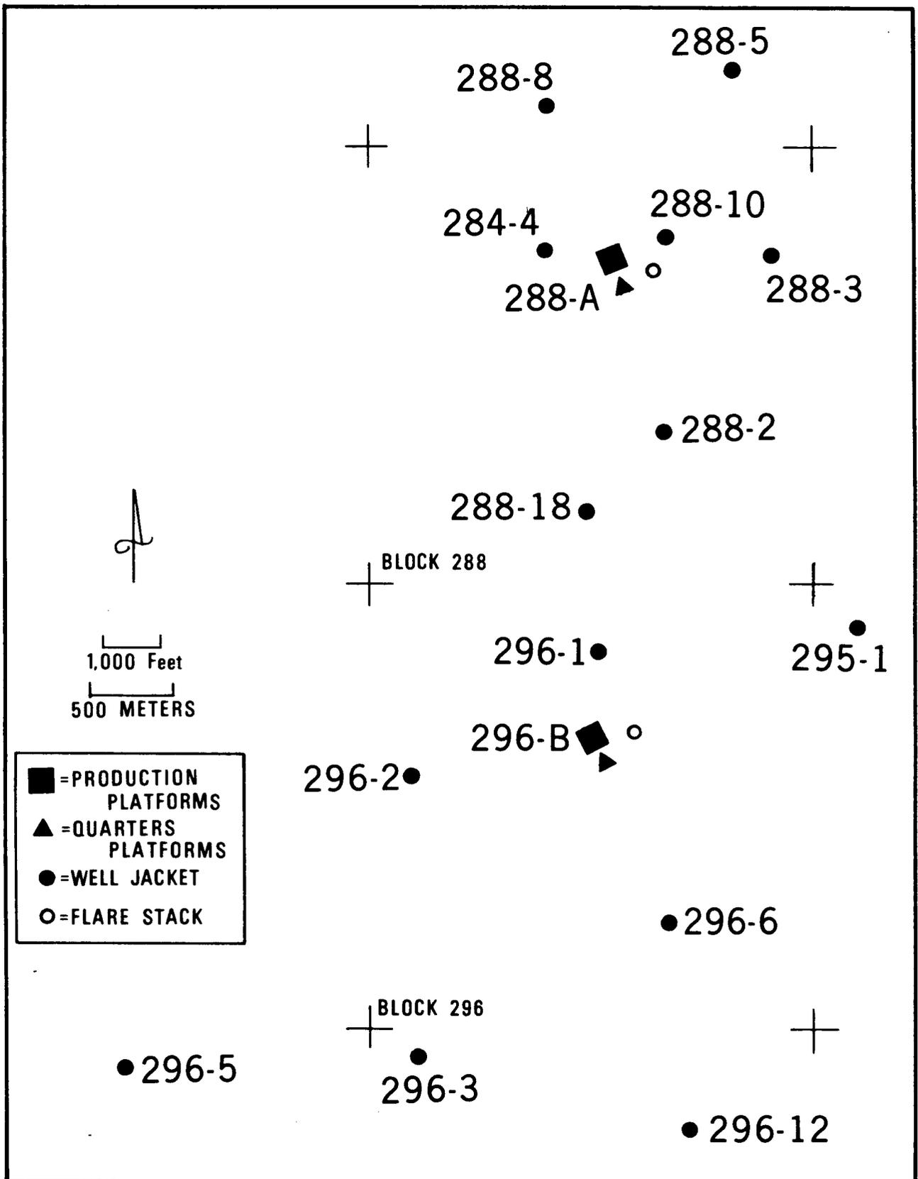
FIGURE 3. SHELL OIL COMPANY'S ALPHANUMERICAL IDENTIFICATION OF BUCCANEER GAS AND OIL FIELD STRUCTURES
