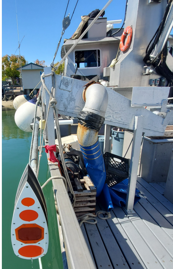
Figure 4: Transducers (Top-bottom: Simrad ES200-7C, ES120-7C, ES38-12, and ES70-7C, Kongsberg) in a pole-mounted multi-transducer array (MTA4) installed on Long Beach Carnage .
