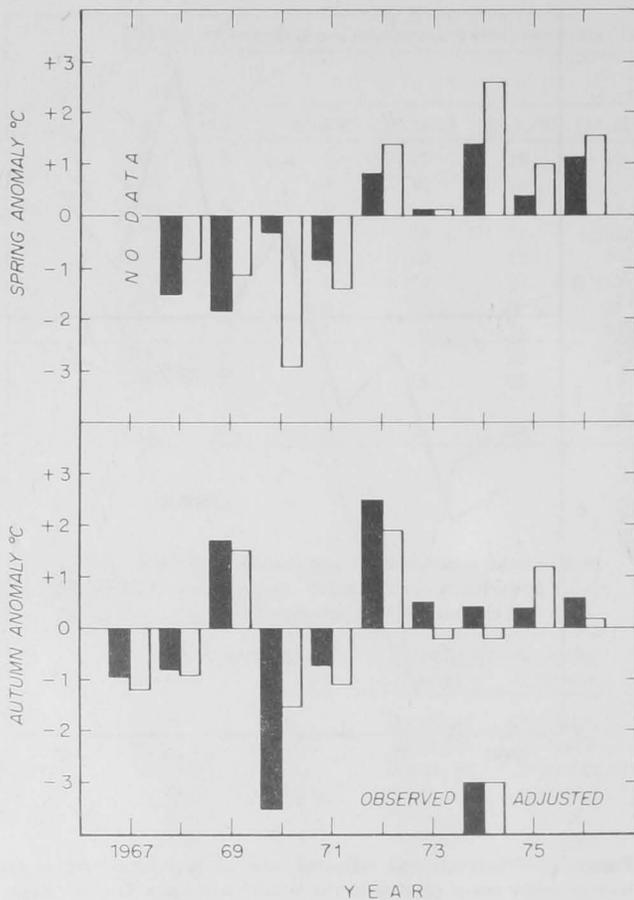
Figure 8.—Observed and adjusted mean bottom-water temperature anomalies in the southern Middle Atlantic Bight during spring 1968-76 and autumn 1967-76. The "O" base lines are based on the seasonal time-series mean temperatures during each season.
