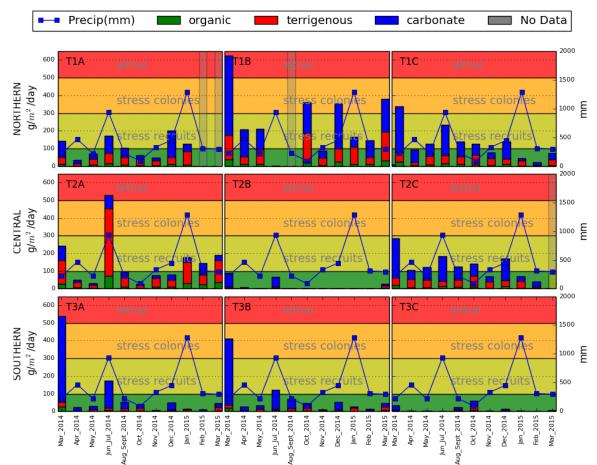
Figure 12. Time series of sediment accumulation in the tubes, March 2014-March 2015. Thresholds vary by coral species but most sources agree sedimentation rates over 500 g/m2/day are usually lethal (Erftemeijer et al., 2012; Fabricius, 2005).
