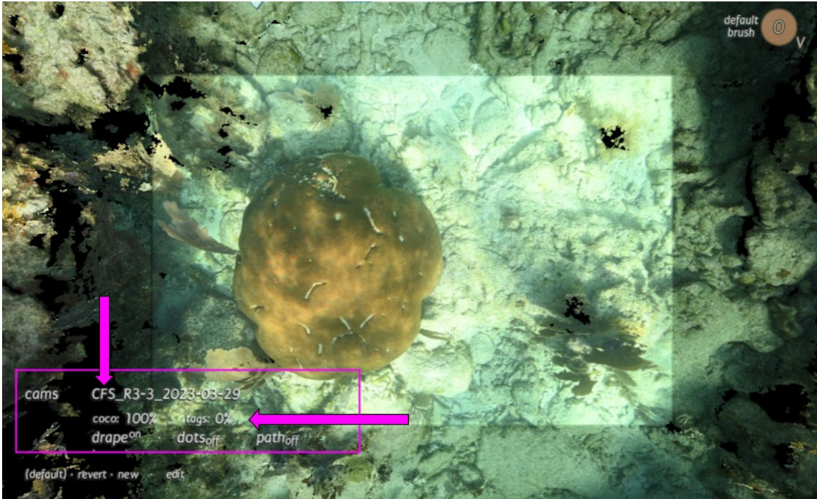
Figure 65. Checkerboard disappears, and the raw image associated with the model area is displayed. Note the Tags menu to change raw image display.
