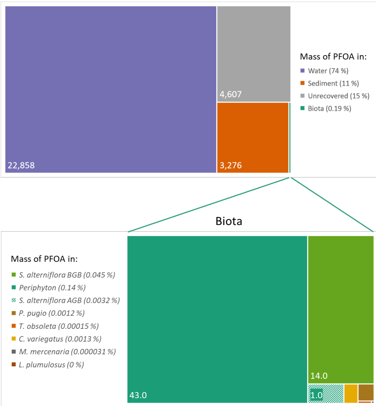
Figure 24: PFOA Mass Balance for the High PFOA (70 mg/L) treatment. The values within each box represent the mass (mg) of PFOS in each compartment and the boxes are sized proportionally relative to one another. The lower box is expanding out the biota compartment of the upper box (BGB = Below Ground Biomass [ S. alterniflora rhizomes and roots], AGB = Above Ground Biomass [ S. alterniflora stems]).
