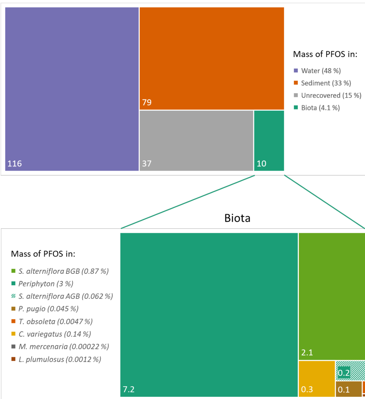
Figure 22: PFOS Mass Balance for the Mixture (0.55 mg/L PFOS / 7.0 mg/L PFOA). The values within each box represent the mass (mg) of PFOS in each compartment and the boxes are sized proportionally relative to one another. The lower box is expanding out the biota compartment of the upper box (BGB = Below Ground Biomass [ S. alterniflora rhizomes and roots], AGB = Above Ground Biomass [ S. alterniflora stems]).
