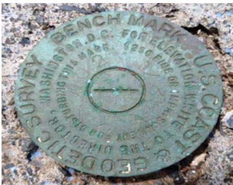
Figure 1. Local Mean Sea Level (LMSL) datum for Lanai is Station 161 4465 TIDAL 2 (PID DL6323) at a height of 3.478 m.
