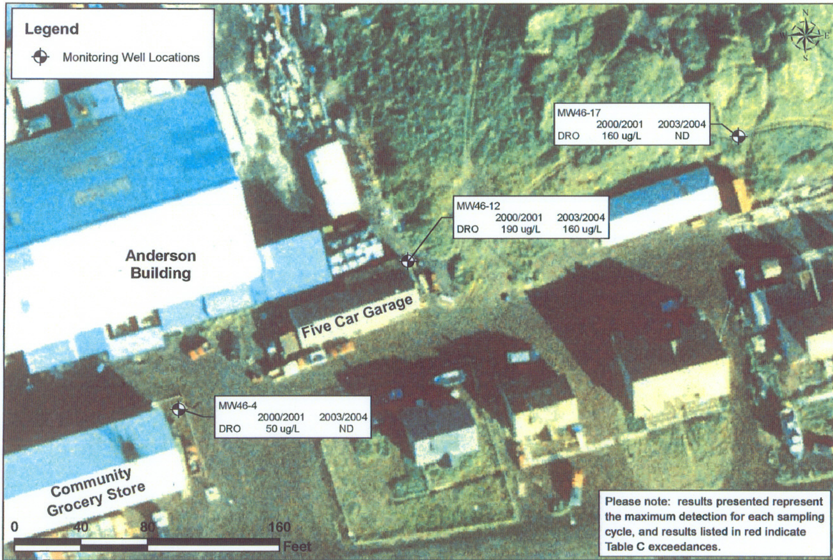
Figure 4 Groundwater Sampling Results Five Car Garage and Anderson Building Site 25/TPA Site 9j St. Paul Island, Alaska Sources: Well Locations (NOAA GPS 2003), Aerial Photo (Aeromap US 1996).
