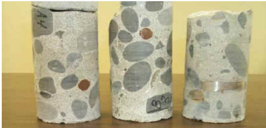
Figure 5. Concrete Cores from the Blubber House Slab
