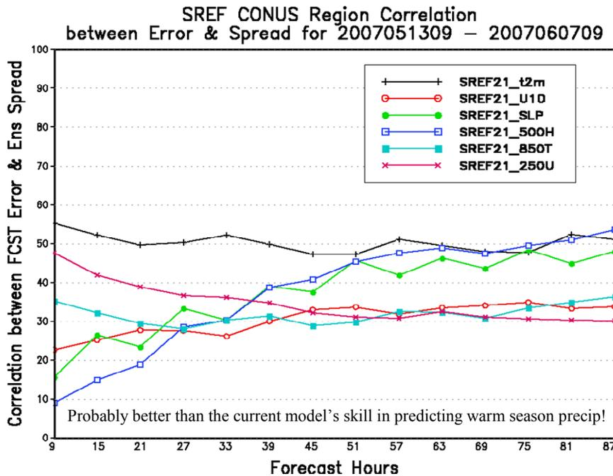
**Figure 10** Spatial correlation (%) between ensemble spread and absolute error of mean-forecast of 9z cycle of NCEP SREF averaged over a period from May 13, 2007 to June 7, 2007 for various forecast variables.
