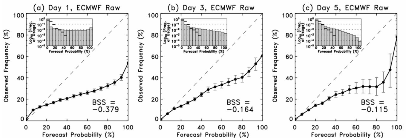
**Figure 5** Reliability score of probabilistic forecast of 12-hourly accumulated precipitation  $\geq 5$  mm over Continental US at day 1, 3 and 5 leads averaged over 480 case days, based on raw ECMWF global ensemble (15 members). It shows over-confident in the probabilistic forecasts. [Courtesy of Dr. Thomas M. Hamill of Earth System Research Lab/NOAA]
