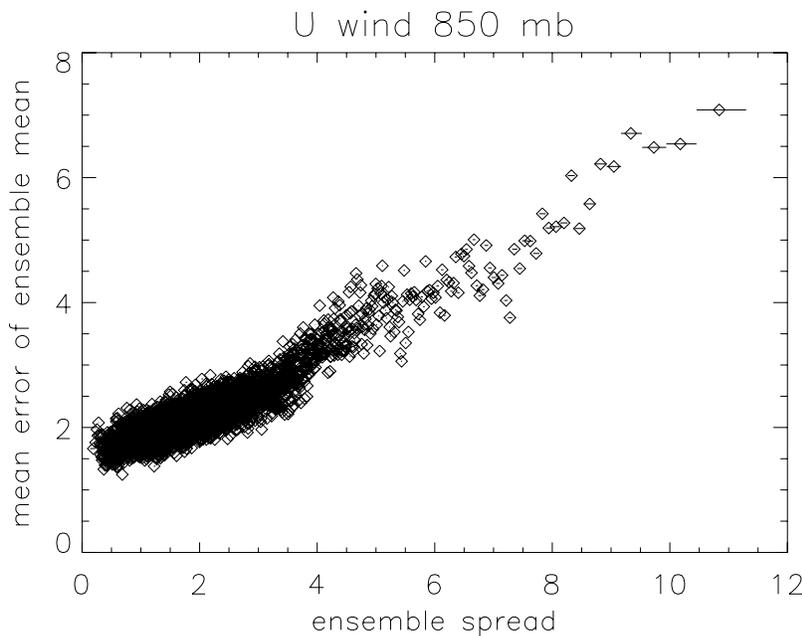
**Figure 8** The spread-skill relationship between ensemble spread and mean absolute forecast error,  $\langle |forecast - verification| \rangle$ , of 63-h forecasts of u component of 850-hpa wind of NCEP SREF. Each point represents the mean error of 1000 forecasts with similar values of ensemble spread. [Courtesy of Dr. Mark S. Roulston of UKMO]
