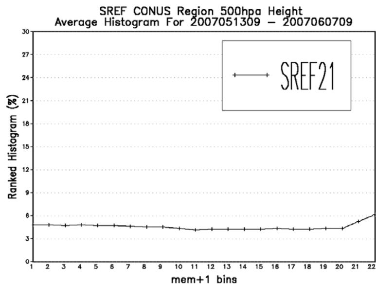
**Figure 11** Talagrand distribution of 500-hpa height ensemble forecasts at 87h lead time averaged over a period from May 13, 2007 to June 7, 2007, based on NCEP SREF data. It indicates slight low bias.
