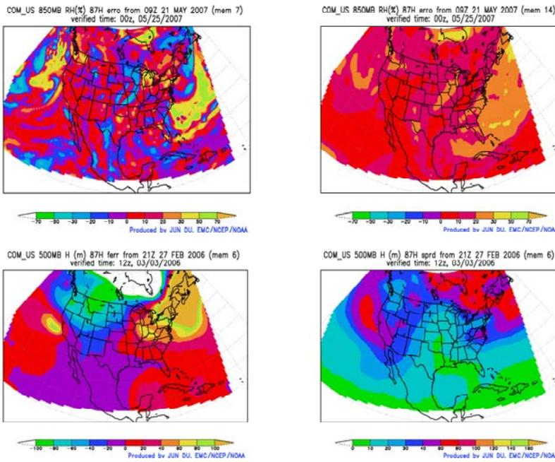
**Figure 9** Two snapshots of spatial distribution of 87-h mean-forecast error and spread from NCEP SREF. Upper panel is for 850-hpa relative humidity initiated at 09z, 21 May 2007. Lower panel for 500-hpa height initiated at 21z, 27 Feb, 2006. Left: error; right: spread.
