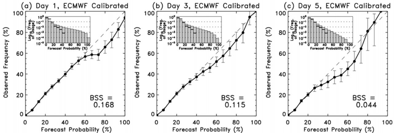
**Figure 6** Same as Fig. 5 but for post-calibrated ensemble with a 20-year weekly 15-member reforecasting ensemble data. It shows much more reliable probability comparing to the raw ensemble-based probability (Fig. 5).
