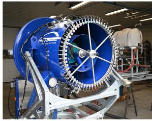
**Figure 4.** The CARI system is similar in design to a snow making device, with an array of nozzles and generated aerosol accelerated by an integrated fan. (Shown here with a sub-set of nozzles 60 in an outer ring only; the system can accommodate a total of 250 nozzles.)
