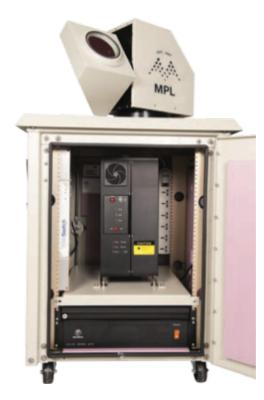
Figure 7. The miniaturized MicroPulse Lidar instrument built by Droplet Measurement Technologies is a widelyused instrument designed to measure tropospheric aerosols.
