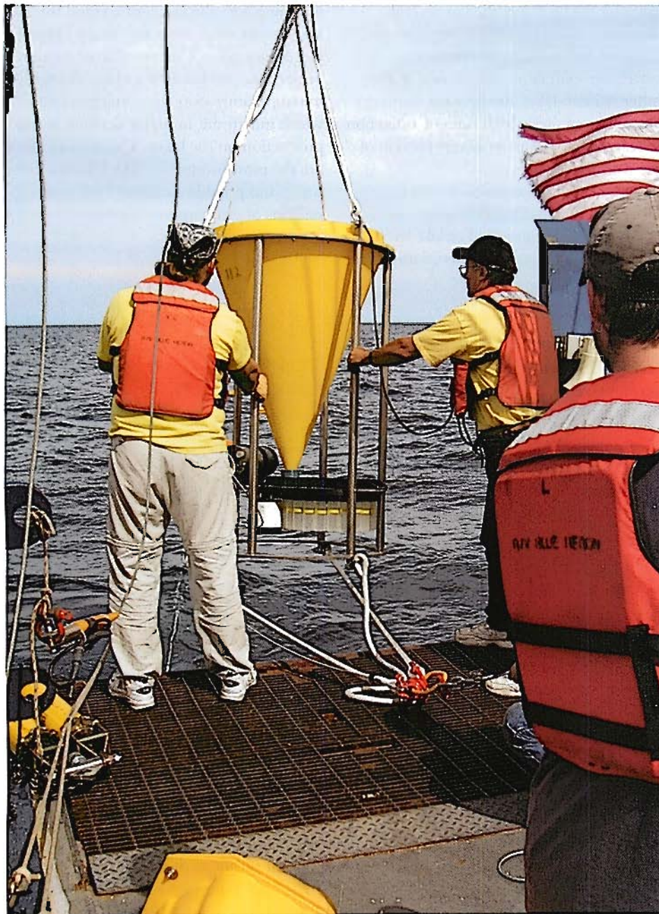
Deploying a sequencing sediment trap in Lake Superior, which will collect particles that sink to the bottom of the lake for six months.
