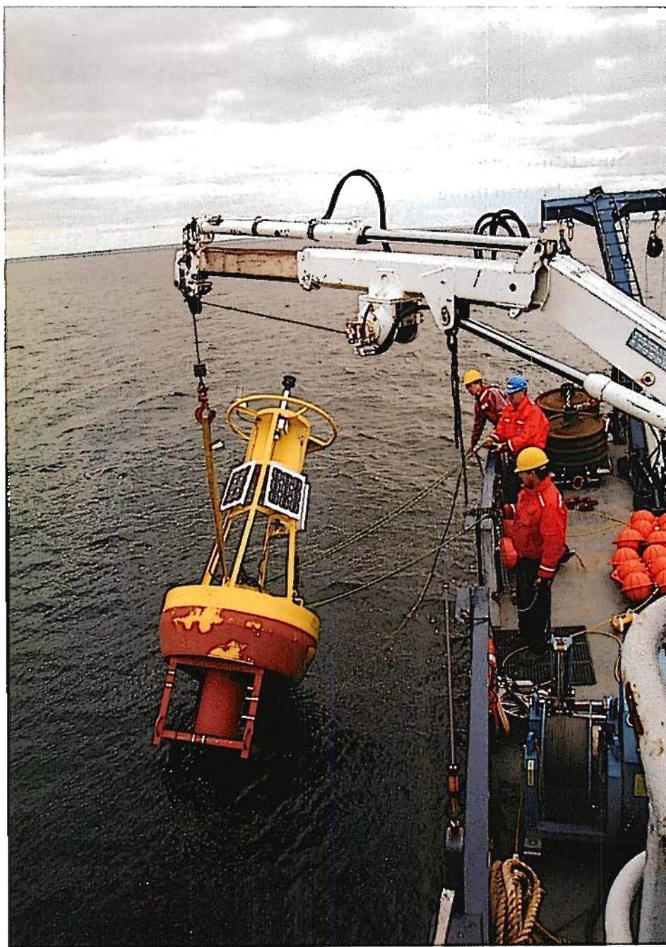
UMD researcher, Jay Austin (top), and his crew carefully lower a research buoy into Lake Superior. The buoy collects weather and water information that will further understanding of the lake's patterns and currents.
