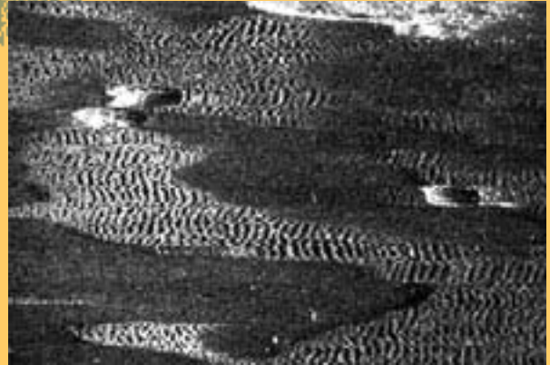
A sandwaves image taken off of Santa Cruz Island by the side scan sonar during the 1999 CINMS SSE.
