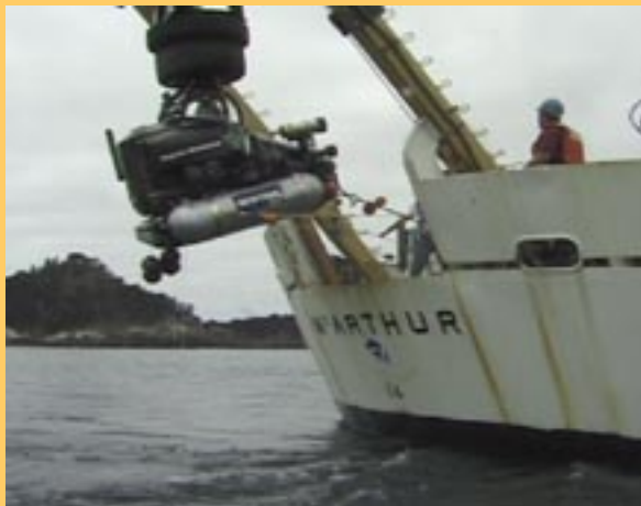
The Deepworker is recovered and returned to the McArthur deck. (Photo courtesy of Kip Evans.)
