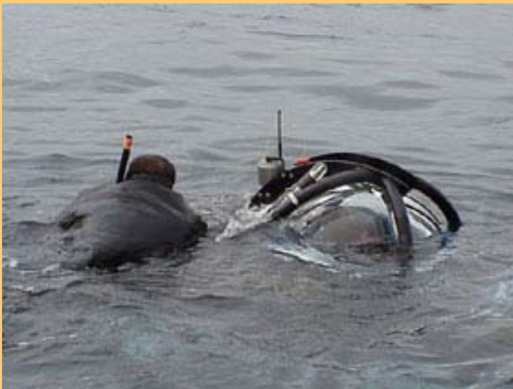
Diver Dana Wilkes releases lines that attach the sub to the ship during launch and recovery.
